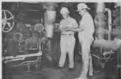
During their survey at Lago, Hygienists Marcos Paoli (at left) and Cesar Azocar from Creole-Venezuela take readings on their instruments on noise level and possible gas release in Powerhouse No. 1. Durante nan investigacion na Lago, Higenistas Marcos Paoli (na robes) y Cesar Azocar di Creole ta midi zonido y posible escape di gas den Powerhouse No. 1.
